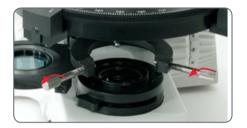
Slide the substage condenser into the fork mount located underneath the stage by aligning the positioning pin on the condenser into the slot on the back of the fork.
